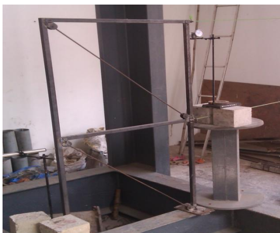
Fig.4 Single bay Frame with Conventional brace
